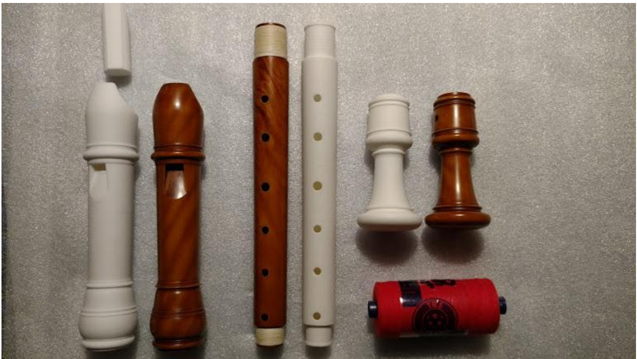
3D Printed recorder parts comparable to a traditionally made instrument
